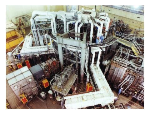
PPPL The Tokamak Fusion Test Reactor at Princeton. TFTR operated from 1982 to 1997, setting many significant records both in plasma temperature and in peak fusion power produced, before it was prematurely shut down.
