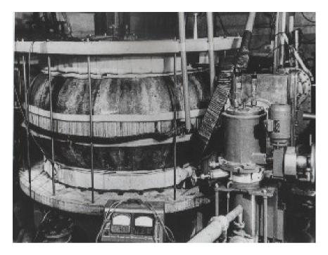
LLNL Basic tokamak design. The tokamak features two external magnetic fields (toroidal and poloidal) designed to contain the plasma long enough for fusion reactions to occur. The first tokamak, T-1, in the Soviet Union.
