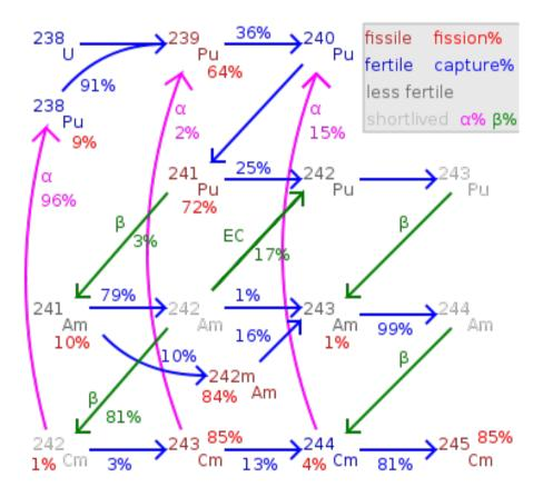
Buildup of heavy actinides in present thermal reactors,[4] which cannot fission actinide nuclides that have an even number of neutrons. Fast reactors can fission all actinides.
